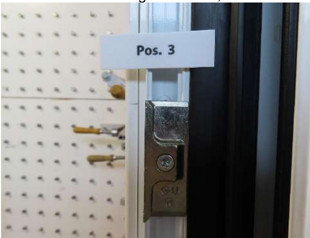
Picture 39 Locking situation 3, inactive casement
