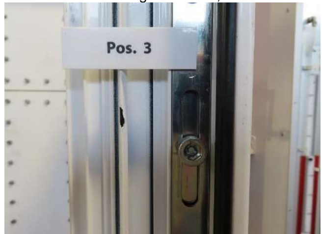
Picture 40 Locking situation 3, active casement
